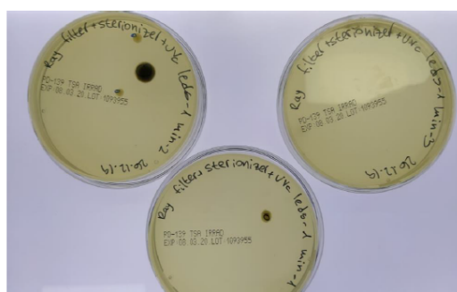
Figure 13: incubation results of the Roy filter+ Sterionizer+ UV-C LEDs plates on December 31 st , 2019
